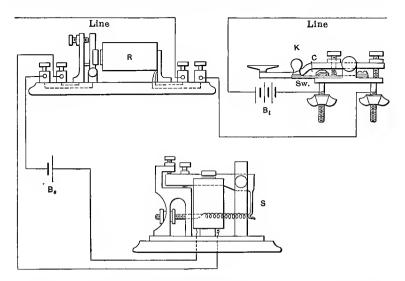
FIG. 10. Simple telegraph circuit showing, R, relay; K, key; Sw. switch; C, contact; Bl., line battery; Bs., local battery; S, sounder.
